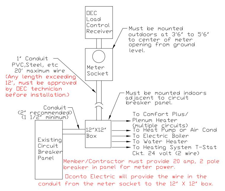
Use only fittings suitable for electrical conduit, <u>NO PLUMBING PIPE OR FITTINGS WILL</u> BE ACCEPTED.
