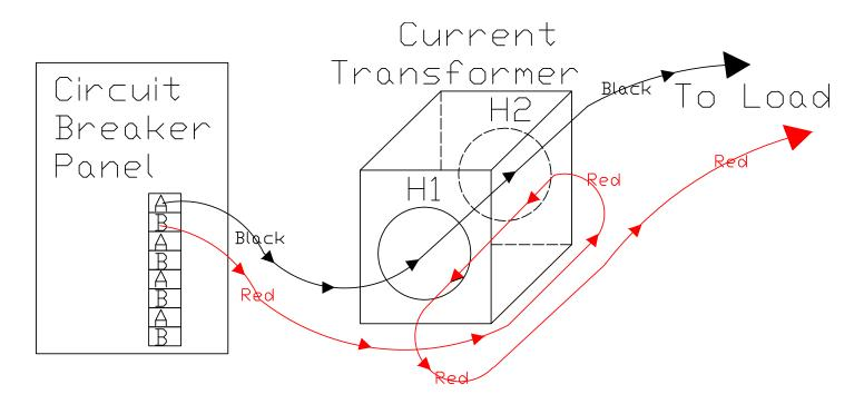
The black wires from Phase A must always be fed through the H1 side of the CT.
